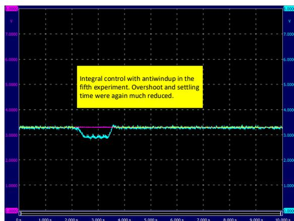
Fig. 11. Tachometer signal in the fifth experiment
